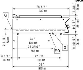
EQ = Equipotential screwG = Gas connection
